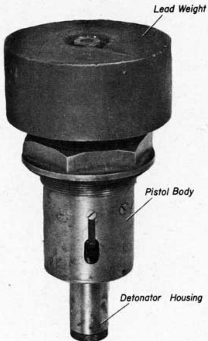
Fig. 7 - Pistol for Tactical Depth Charge.
